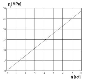
Fig. 6. The caracteristic of the disconect valve.
