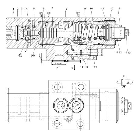
Fig. 3. The disconnection valve suggested proposed.
